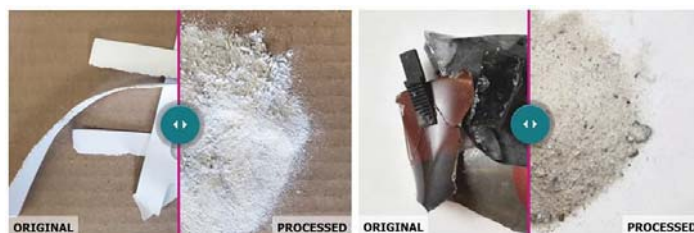
Ceramic strips before and after being processed by a hammer mill.
