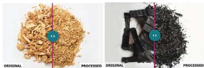
Wood chips before and after being processed by a screen classifying cutter.
