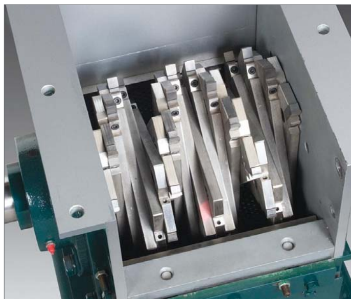
This closeup of a screen classifying cutter illustrates a helical array of carbide-tipped holders that continuously shear material against twin, stationary bed knives.
